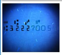
Checks printed with TROY UV MICR Toner appear as standard black ink to the naked eye but fluoresce blue under UV verification light. Authentication is achieved when the document is held under a UV light. providing an additional layer of covert security and authentication.
